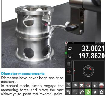
No need to hold the crank handle during this operation. In motorized mode, diameter measurement is performed automatically in a single operation. The reversal points is clearly indicated by audible and visual signals. The user is thus guided precisely during diameter measurement, which results in a significant increase in speed and reliability of the result.
