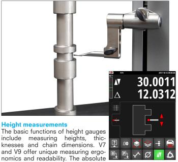
dimension (=from zero) and the distance from the last probe are displayed at the same time for each measurement. This allows a very efficient measurement of chain dimensions. All results are displayed in the buffer as a list. The toleranced dimensions are displayed in colour according to the result.
