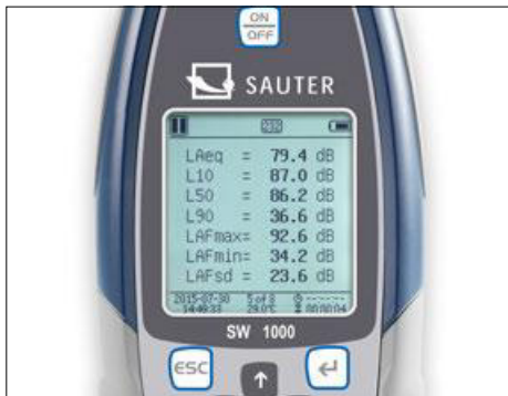
Data logging function with date and time in the device...
