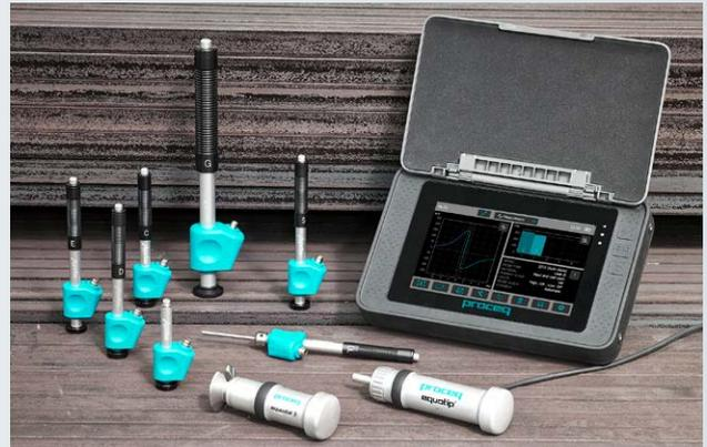
The **Equotip 550 Portable Rockwell** is a static hardness measurement solution which is highly appreciated for applications on thin or light samples. Furthermore, it can be used on almost all materials without special adjustments, which also makes it popular to use as a reference method for other measurement principles. A wide variety of accessories makes it very versatile.
